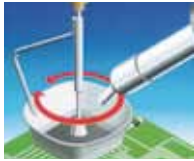
Desoldering IC component with hot air
