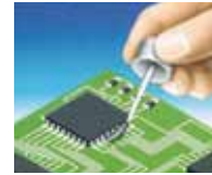
Fluxing IC pads and leads
