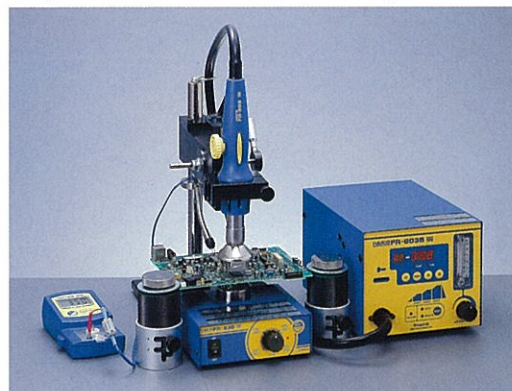
Setting example:FR-803B, C1390C (Omnivise), C1392B (Rework fixture), FG-100 and C1541 (Temperature probe) with FR-830
